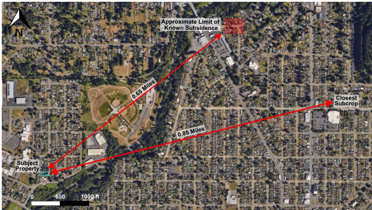
Site plan showing the subject property and the distance to the nearest known zone of historic subsidence and the closest location underlain by the subcrop.
